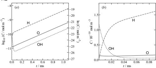
The figures show the numerical solution for the rate equations for reactions 1–3 for the 2:1  $H_2$ - $O_2$  mixture at T = 1000 K, p = 1.01 kPa,  $[O]_0 = 1.46 \times 10^{-11}$  mol m<sup>-3</sup> and  $[OH]_0 = 1.22 \times 10^{-10}$  mol m<sup>-3</sup>. The coefficients for the solution (7.2) at this condition are shown below.
